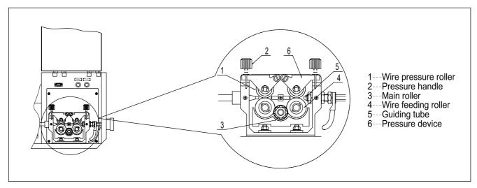
Fig. 4-9-5: Wire feeder structure
