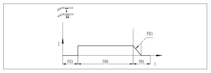
Fig. 4-3-8: Spot welding mode
