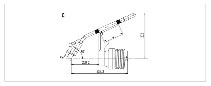
Fig. 4-6-2: Different buckling angle for robot torch neck
