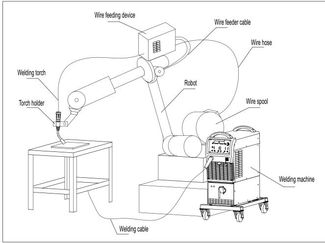
This series inverter welding machine is specially designed for working with robot, it needs follow parts to combine robot welding system.
