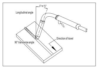
Fig. 7-1-4: Butt & horizontal welds
