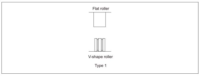
Type 1: for hard wire, such as carbon steel wire, stainless steel wire
