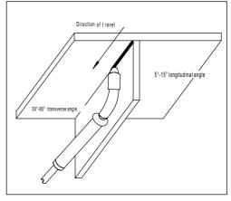
Fig. 7-1-7: Overhead weld
