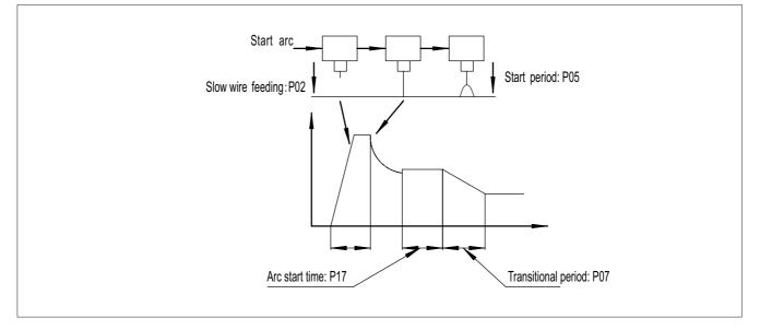
Fig. 4-3-11: Operating mode sequence diagram of start arc
