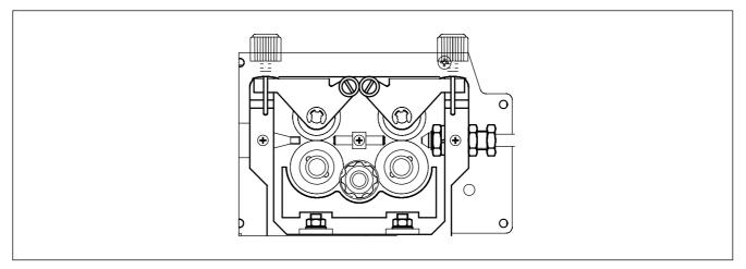
Fig. 4-5-1: Wire feeding device
