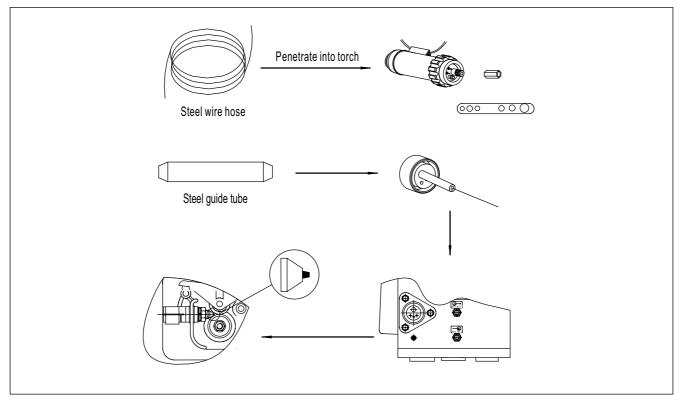
Fig. 4-9-9: Installation of steel wire hose
