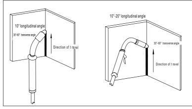
Fig. 7-1-6: Vertical fillet welds
