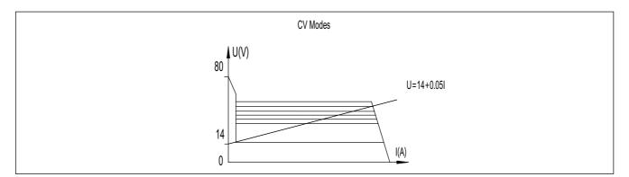
Fig. 1-3-1: Output characteristics
