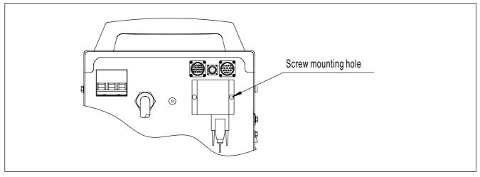
Fig. 4-9-7: Robot interface box installation
