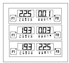
(1) With the "CALL" button (4), indicator (22) is on -the last job used is displayed. To view settings programmed in this job, use the "Parameter selection" buttons (2) and (3). The process and operating mode of the stored job are also displayed.
