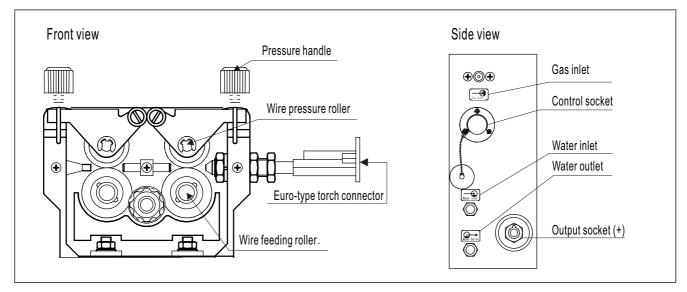
Fig. 4-5-2: Wire feeding device interface
