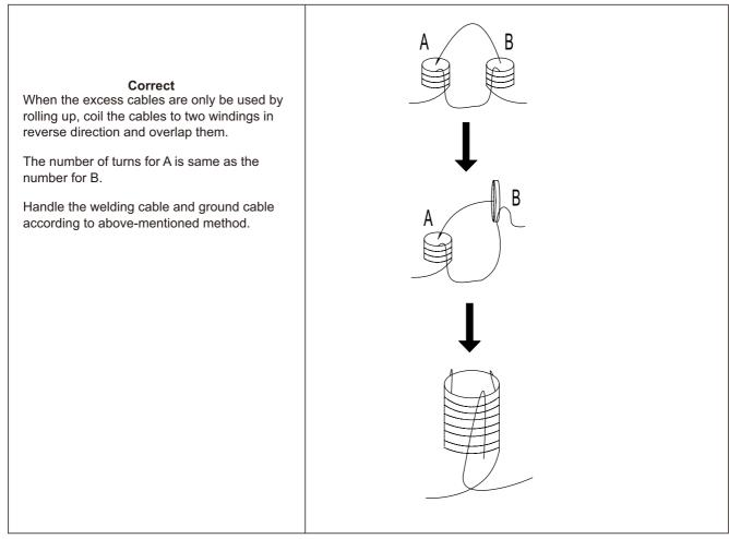
Fig. 3-4-1: Welding cables instruction
