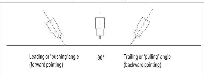
Fig. 7-1-10: Nozzle Angle Right Handed Operator
