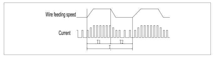
Fig. 4-3-9: Double pulse wave form
