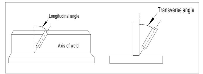
Fig. 7-1-9: Transverse and Longitudinal
