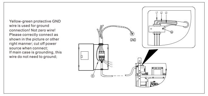
Fig. 4-9-1: Connections for input cable and distribution box
