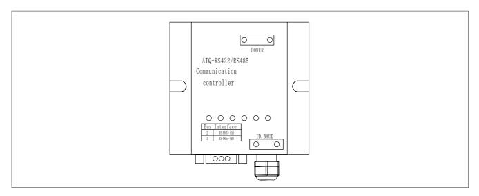
ATQ-RS422/RS485 interface box adopts standard ModBus RTU method to output data.
