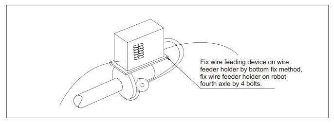
Fig. 4-9-3: Installation for wire feeding device
