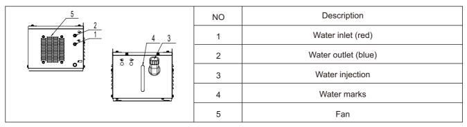
Fig. 4-8-1: Water cooling system connections
