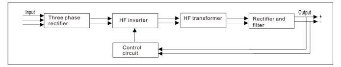
Fig. 1-2-1: Schematic diagram
