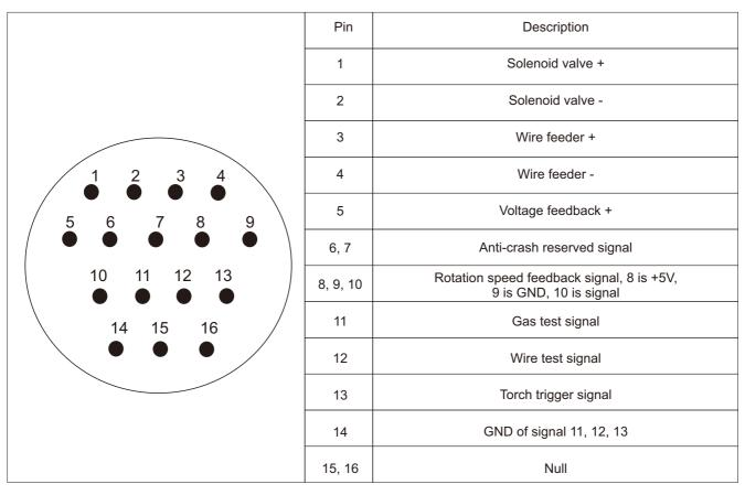
Table 4-4-3: Wire feeder control socket X7
