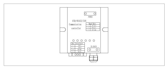
Fig. 4-7-5-1: ATQ-RS422/CAN interface box
