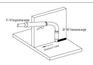
Fig. 7-1-5: Horizontal fillet weld
